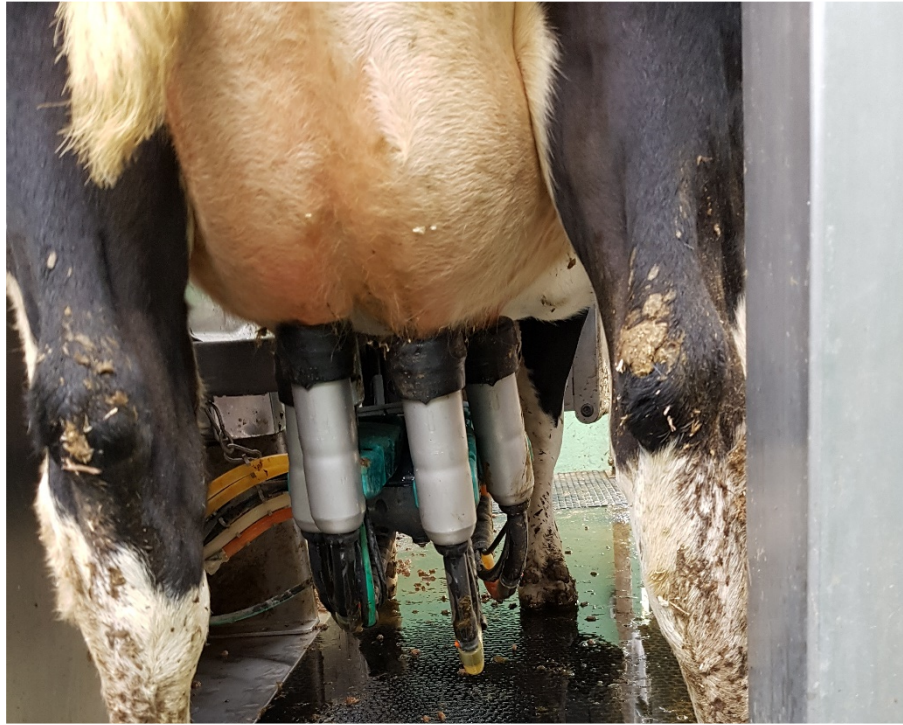
Figure 16: Robotic milking system in the South West Dairy Centre; source Agri-EPI centre
