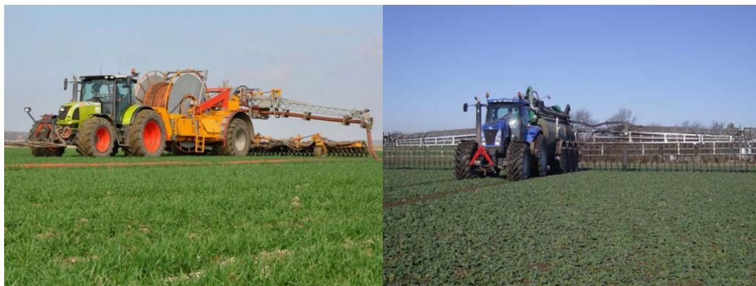
Image 8: Application of slurry to arable crops using modern low impact equipment
